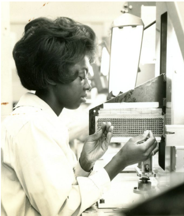
A worker programming Core Rope Memory (Transistor Museum.)
